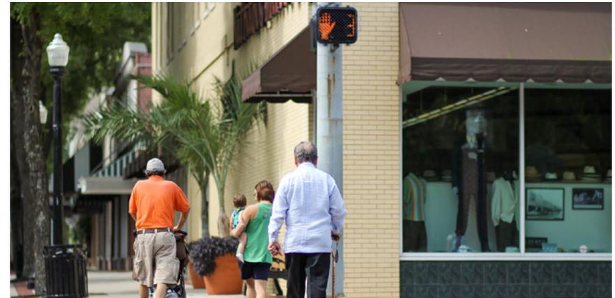
A Pedestrian Countdown Signal provides visual information on the number of seconds left to safely cross the roadway before the light changes and vehicles can enter the intersection. The countdown time is based on walking speed and crossing distance. For instance, an eight-lane roadway would have a longer countdown period than a four-lane roadway because of the longer distance to cross. The following safety information will help you properly use this pedestrian signal.
